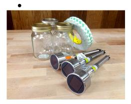
STEP 1: Remove stake piece of the light (this just pulls off) so you are left with the top solar panel piece. Keep the plastic casing around the light because it has a metal reflector that helps intensify the brightness of the lamp.
